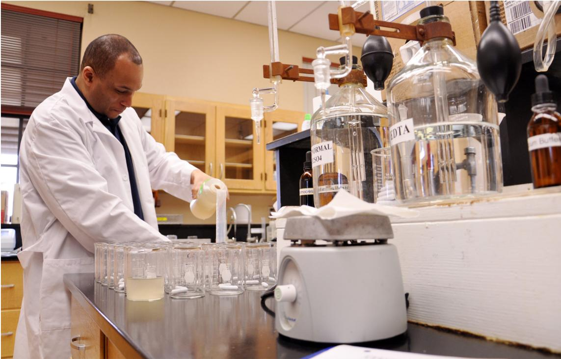
taffed by chemists, microbiologists and technicians, the Sewerage and Water Board Water Quality Laboratory assures the safety and purity of the city's water by testing for some 150,000 organic, inorganic and microbiological compounds. The 8,500 square foot lab is located within the Carrollton Water Plant and monitors river water and finished water sampled from both the East Bank and Algiers. Pictured here, a Laboratory chemist performs water analysis.
