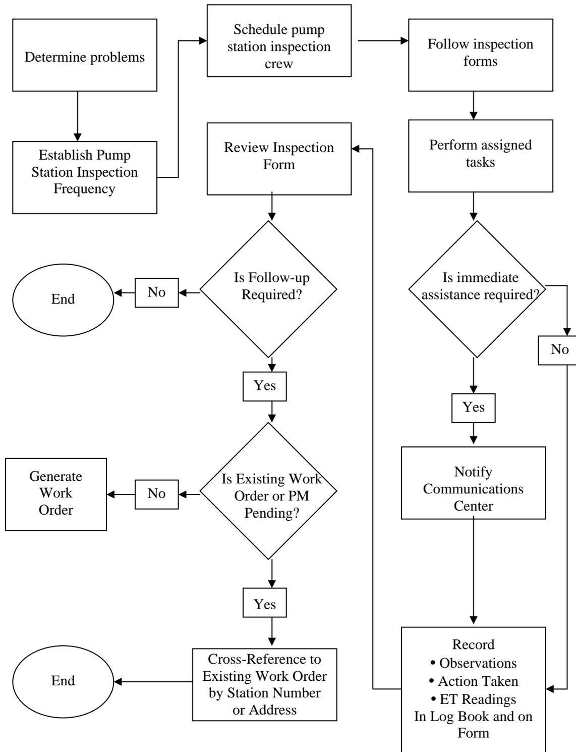
**5.1.2 - Sewage Pumping Station Inspection Form:** Sewage Pumping Station Maintenance Inspectors follow a comprehensive checklist.
